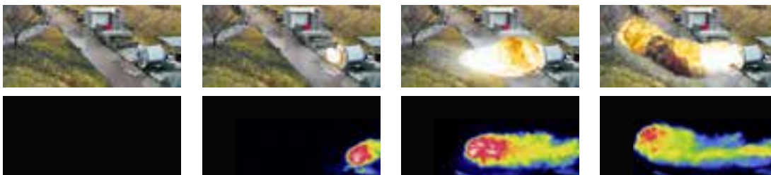
Thermographic investigation of a dust explosion: conventional explosion venting with an explosion vent.
