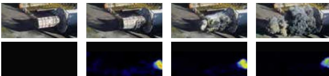
Identical explosion with the Q-Rohr®: no heat generated outside the vessel with only a slight pressure rise and minimal noise volume.
