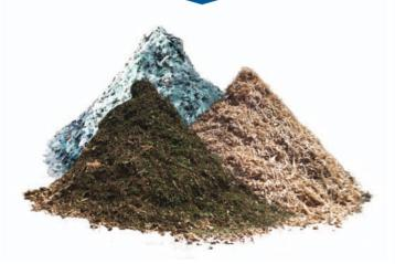
Final grain: approx. 200mm 4-fold fracture- and cutting-process in one shaft rotation
