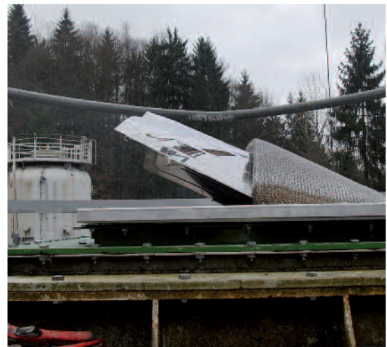
After an explosion and venting: The TARGO-VENT technology limits the relief angle of the explosion panel.
