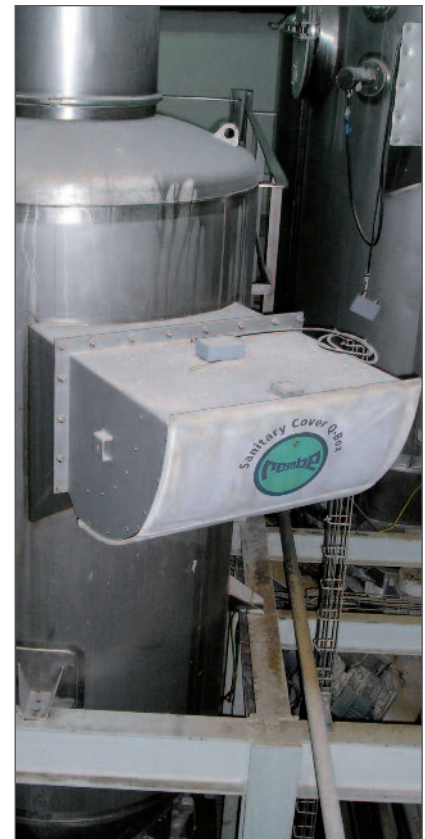
Q-Box II application in the food industry: the sanitary cover protects the exterior of the Q-Box II; keeping it clean from the outside
