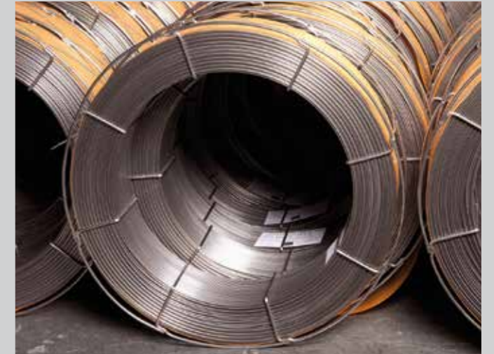
VAUTID hardfacing material as tubular wire
