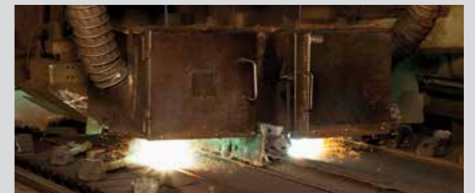
Production of VAUTID wear plates
